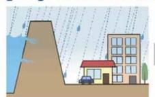
When river water increases during heavy rain, water pressure is applied to riverbanks.
